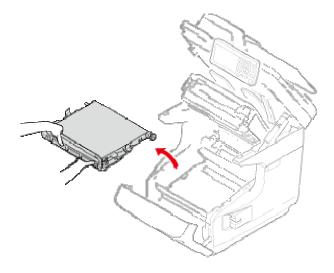
9. Hold the handle of a new belt unit with your hand and support lower part with other hand. Set the belt unit into the machine.
