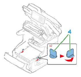
8. Remove the belt unit by holding the blue lever.
