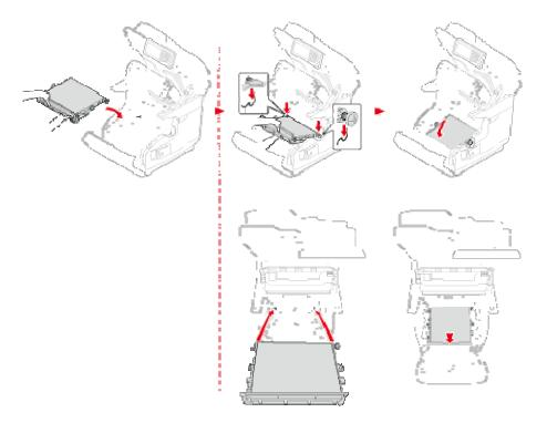
**10.** Turn the blue locks (4) on each side of the belt unit in direction of the arrow.
