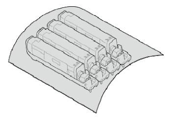
7. Turn the blue locks (4) on each side of the belt unit in direction of the arrow to unlock.
