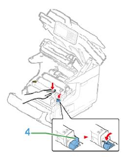
7. Lift the toner cartridge (5) from right side, and remove it from the machine.
