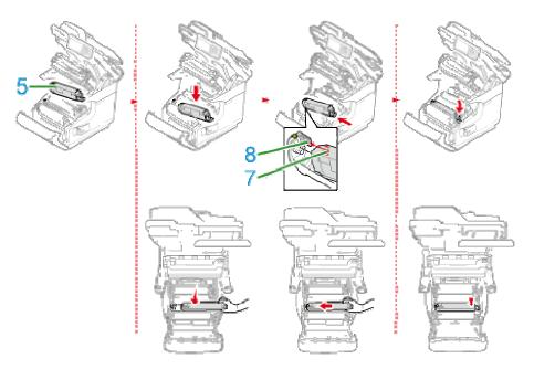
12. Turn the blue lever (4) of the toner cartridge backward until its top align on the mark while pressing the toner cartridge.
