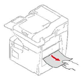
3. Check for jammed paper in the duplex unit. If jammed paper remains, pull it out gently. Check the back side of the duplex unit and remove jammed paper gently if it remains.
