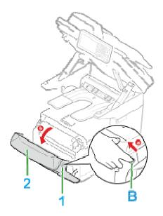
4. Remove the jammed paper gently in the direction of the arrow if an edge of jammed paper can be seen, and then go to step 11. If you cannot find jammed paper, go to step 5.
