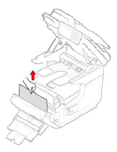
Remove the paper from the back gently if the edge of paper cannot be seen.
