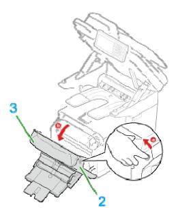
5. Remove the jammed paper gently by pulling the edge of paper.
