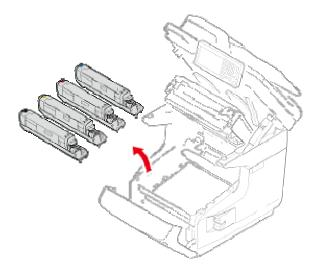
6. Cover the removed image drums with paper so that the image drums are not exposed to light.
