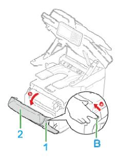
4. Remove the jammed paper gently in the direction of the arrow if an edge of jammed paper can be seen.
