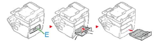
7. Check for jammed paper inside the machine. If jammed paper remains, remove it.
