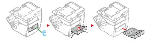
2. Check for jammed paper inside the machine. If jammed paper remains, remove it.
