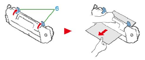
11. If jammed paper remains in the machine, hold the both sides of the paper to remove it gently.
