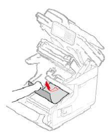
Pull out the jammed paper gently while lifting the release levers (4) on the fuser unit if an edge of jammed paper cannot be seen.
