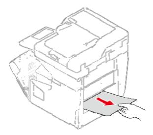
8. Check if paper remains in the duplex unit. If jammed paper remains, pull it out gently. Check the back side of the duplex unit and remove jammed paper gently if it remains.
