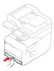
4. Insert your finger into the lever (B) on the right side of the machine and pull the front cover open lever (1) to open the front cover (2) forward.
